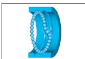
Fig 3.5 Circuit for internal return cap
