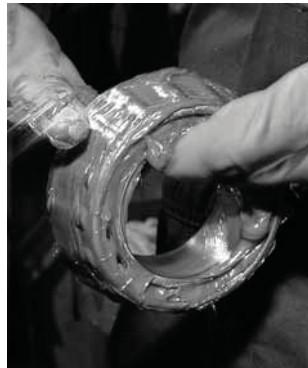
Fig. 14. Grease can easily be packed by hand.
